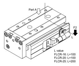
Plate (material: Iron) is attached when measuring. w=12, t=19
