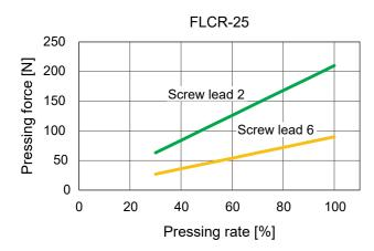
\* Pressing force and pressing rate indicate a guideline. Individual motor differences and variations in mechanical efficiency may result in errors even at the same pressing rate.
