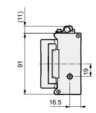
In case of connector outlet direction L (left side)
