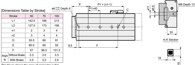
This figure shows the case of connector outlet direction R (right side).
