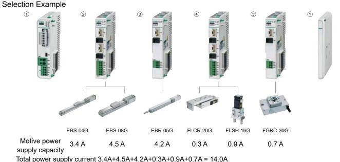
Total 14.0 A (total motive power supply current for batch wiring method) ≤ 30 A ... OK ECG
