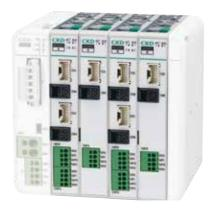
This is a unit that drives an electric actuator. There are units that connect one axis to one drive unit and units that connect two axes. In addition, there are two types of drive units, A-type and B-type, and the actuators that can be connected are different. It is also possible to supply motive power directly to the drive unit. Up to 8 drive units can be connected per communication unit. For details, please refer to P. 548.
